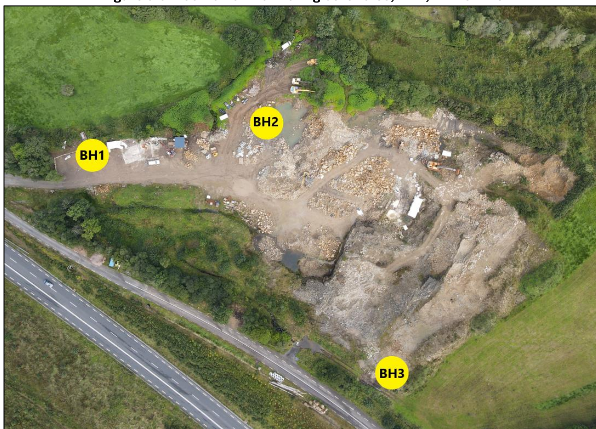
Figure 8.6: Position of monitoring boreholes, BH1, BH2 & BH3
